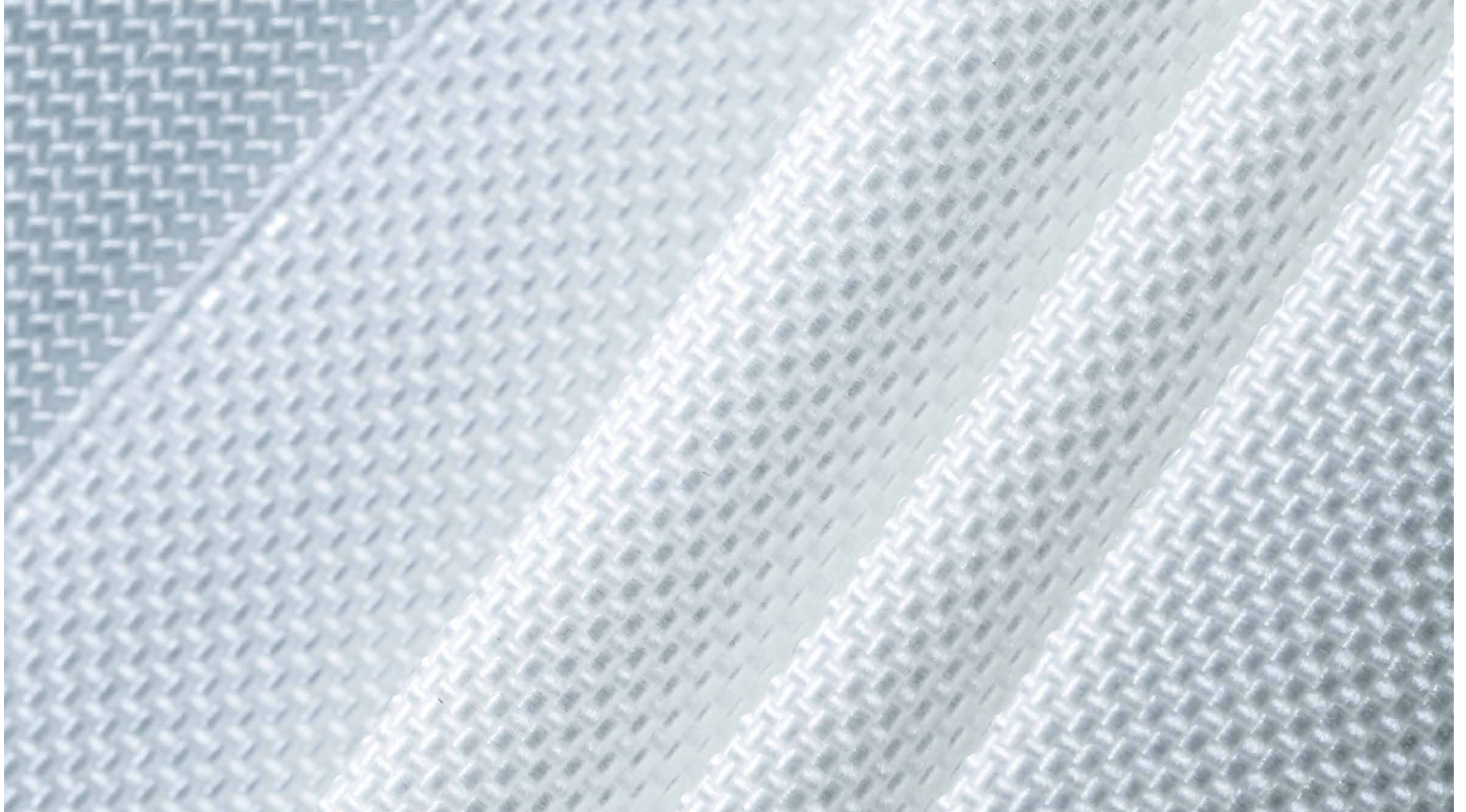
Commercially available airbag fabric. The distinct textile weaving structure is clearly visible.
