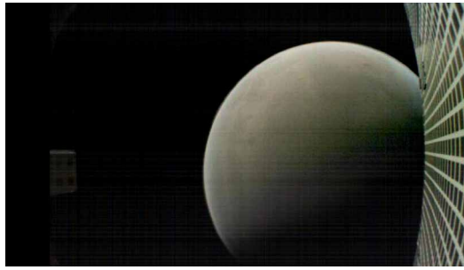
Mars image taken from MarCO-B, a JPL-built 6U nanosatellite with 13.5 kg mass. Two of these CubeSats have been successfully used for relaying the radio link of the InSight spacecraft after landing on Mars surface. © NASA
