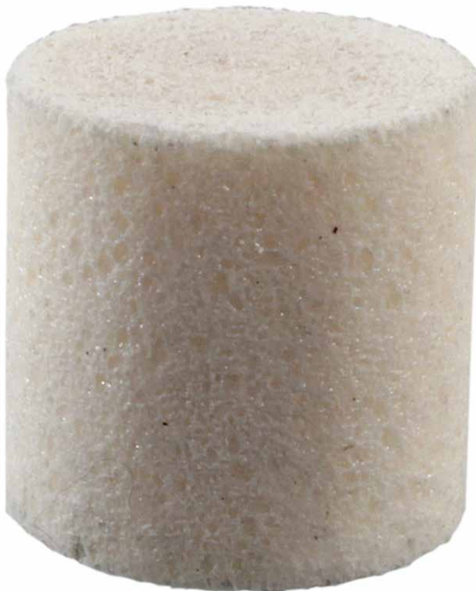
PPX sample for material characterization.
