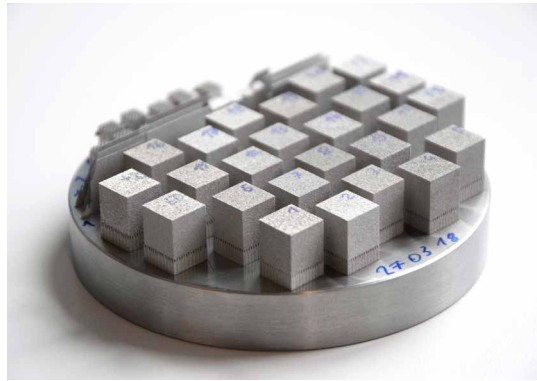
Additively manufactured samples made from heavy metal (tungsten) for the investigation of optimized process parameters.
