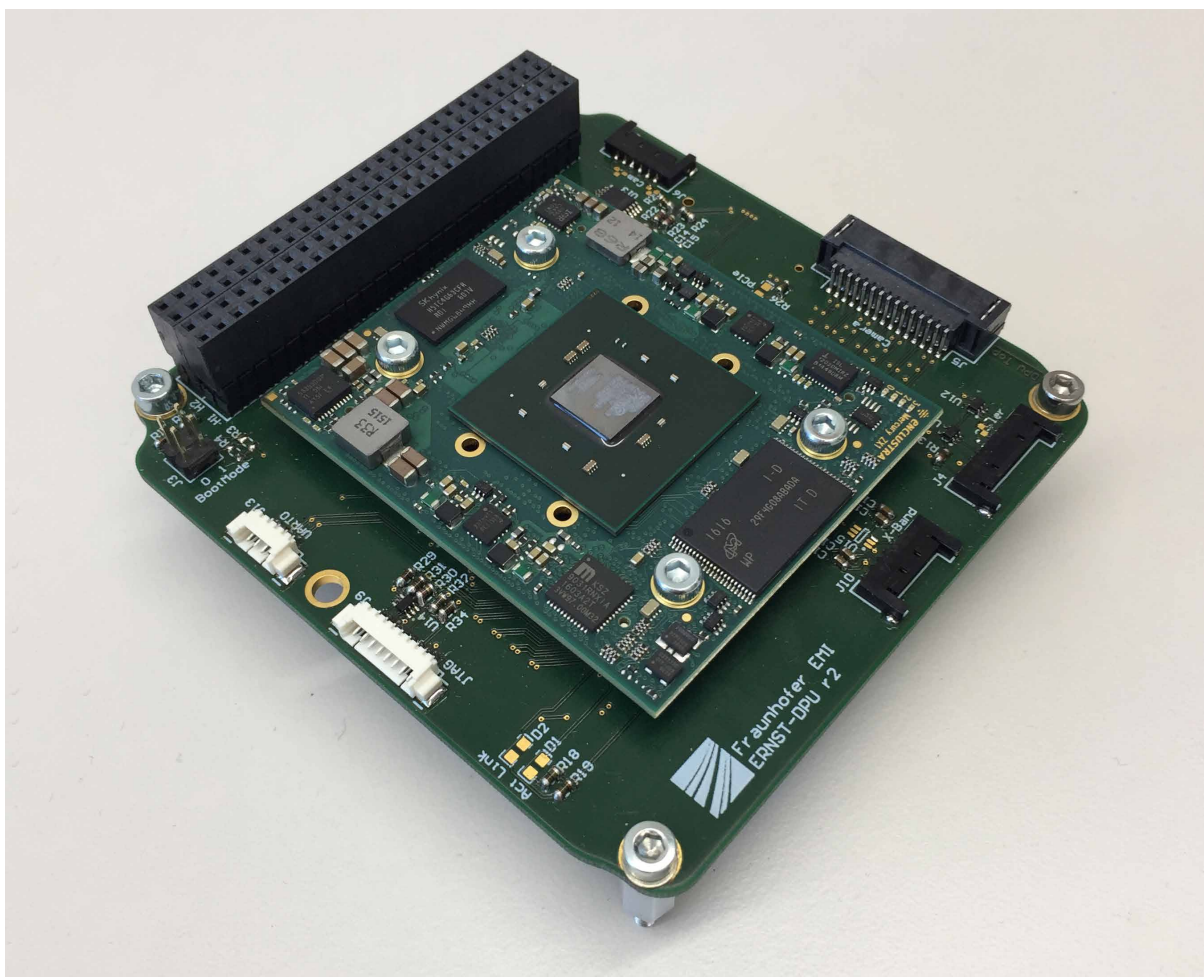
Data processing unit with FPGA technology.
